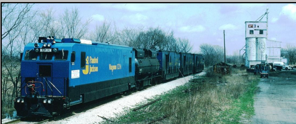
Left: A Pandrol-Jackson (ex-Speno) rail grinding train glides by the Litchfield elevator headed toward Spencer in a probable repositioning move. This mid-1990's view shows the Litchfield elevator, which had ceased rail shipments in 1970. The four concrete silos were erected in 1947 to hold increased wheat harvests. Frank Novak
