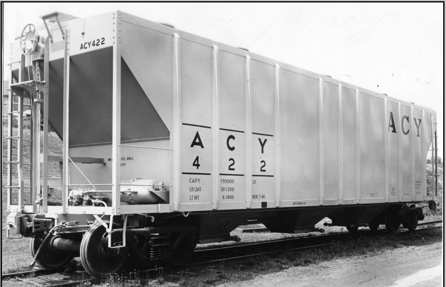
Above: Another great “B-end” view of AC&Y’s PS-2CD 4427 covered hopper number 422. Courtesy Jim Kinkaid
